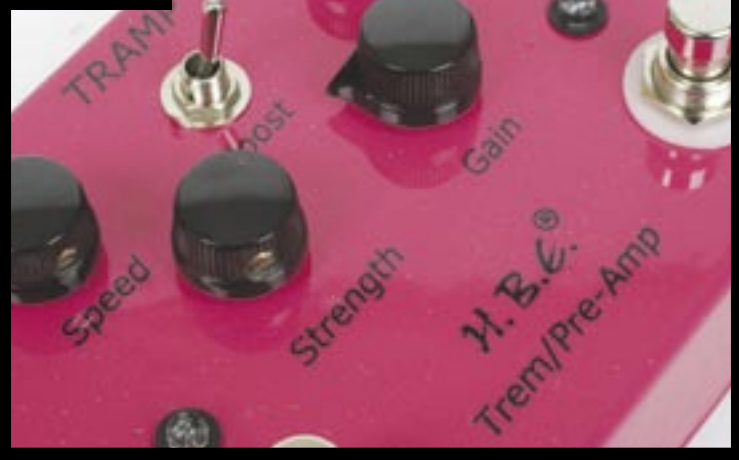
■ The HBE Tramp features speed, strength, gain, level and boost controls
